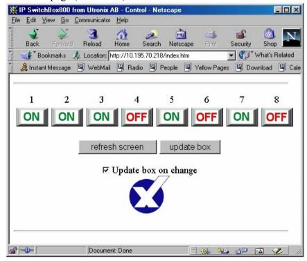
When you click at the ON or OFF button a request for this is sent to the box. Then the button turns gray until the box has confirmed the change. When the confirmation arrives the button indicates current setting again. In this way you can be sure that the change request actually has reached the box and been serviced.
