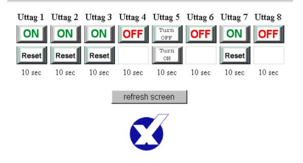
On outlet 5 a reset is started. The Reset can be cancelled by clicking "Turn ON" or "Turn OFF".
