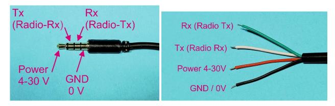
Tx from radio shall be connected to Rx on Aviation Companion and vice versa.
